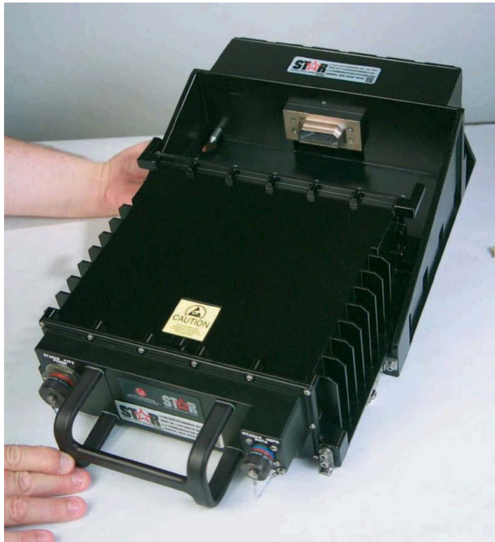
L-3 Communications Systems' RM-3000F solid-state recorder, the standard data recording tool for F-16 podded reconnaissance missions.
